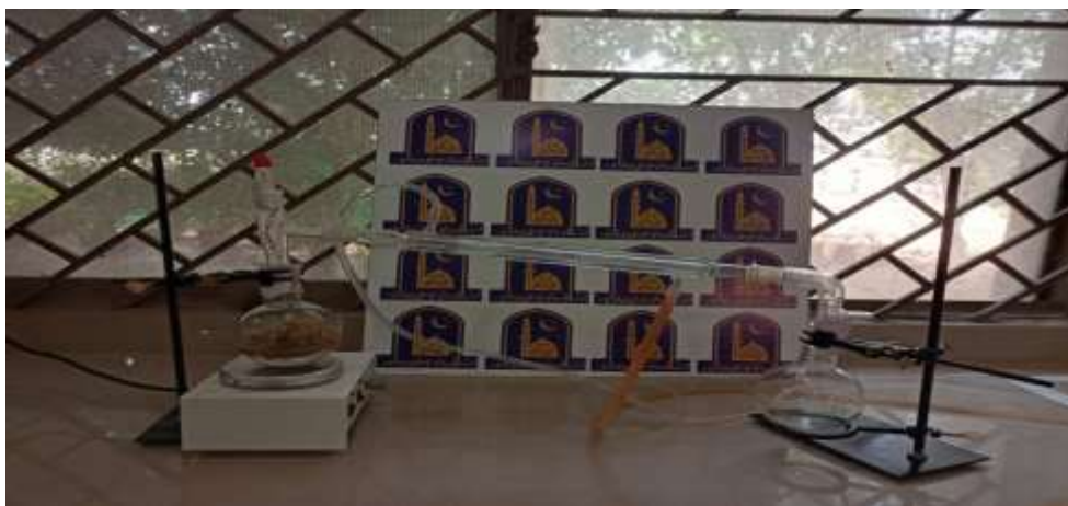
Figure 3.2: Experimental Setup for Furfural Formation
